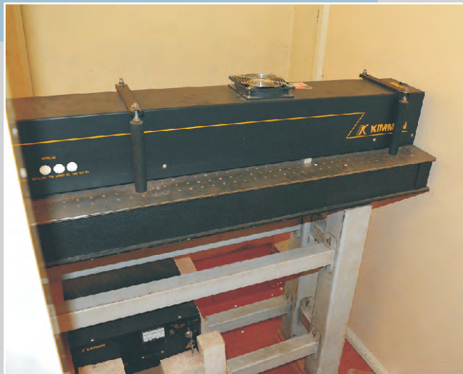
Neon laser, 8'X4' Honeycomb Table Isolation support, Opto-mechanical Components, Optics and Online UPS
